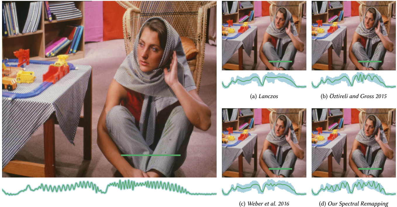
Fig. 1. Comparison of various image-downscaling techniques. (left) Reference image. (right) Downscaling to 180 \times 144 pixels performed with: (a) Lanczos filtering followed by resampling using a cubic B-Spline causes structured high-frequency details from the pants, scarf, books, and most of the table cloth to be removed. (b) The technique by Öztireli and Gross introduces aliasing artifacts in those regions. (c) The technique of Weber et al. removes most of these high-frequency details, but still exhibits aliasing (e.g., see books). (d) By remapping high frequencies to the representable range of the downsampled spectrum, our approach retains the structured details. The green plots under the images are the intensity values of the highlighted pixels. The light-blue envelopes show the horizontally-compressed plot of the reference image. “Barbara” test image attributed to Allen Gersho (public domain). Please zoom in to see the details.
