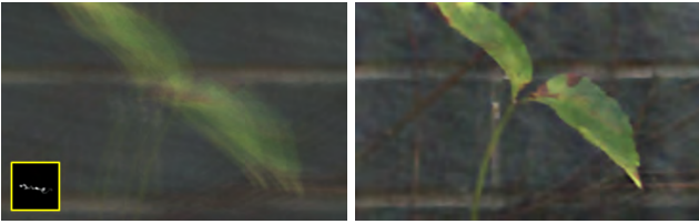
Fig. 9 Example of camera-motion deblurring. (left) Blurry photograph with corresponding camera-motion kernel (shown as an inset) provided by Shan et al.'s [26]. (right) Deblurred result produced by our technique. Note the clearly visible edges and spots on the leaves.
