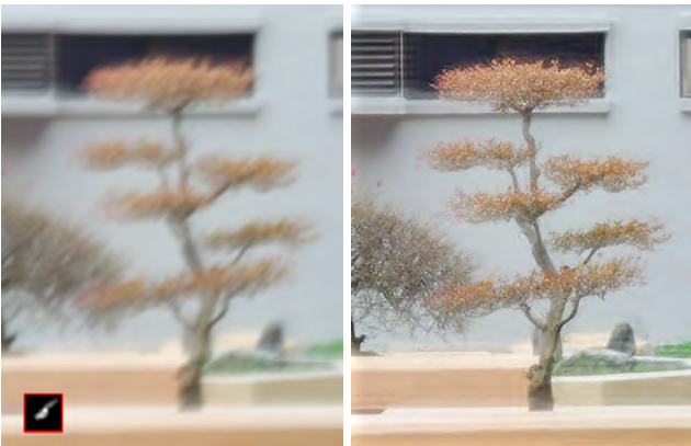
Fig. 10 Another example of camera-motion deblurring. (left) Input photograph and camera-motion kernel pair (by Shan et al [26]). (right) Recovered image obtained with our technique. Note the considerable improvement in sharpness.
