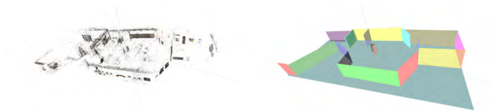
Fig. 1: Example of plane detection using our technique. (left) Museum dataset: point cloud consisting of 179,744 samples obtained from a set of photographs using SynthExport and Photosynth. (right) Planes automatically detected by our technique in just 0.025 seconds on a 3.4 GHz PC. They were manually resized to better represent the original model.
