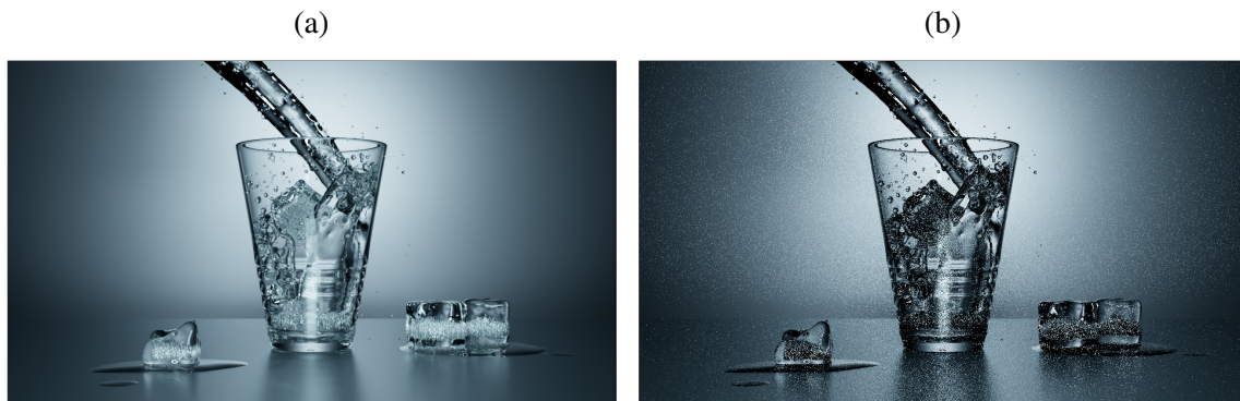
Figure 2.4: Typical noise in an image rendered with a Monte Carlo technique. (a) Reference image. (b) Noisy image rendered with 16 samples per pixel.
