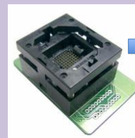
Prototype adaptor board for eMMC mounted at DRAM BIB
