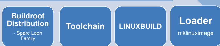
Figure 1. Linux Cross-compilation Workflow: The blocks necessary to achieve the linux boot image.
