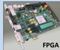
Prototype FPGA board to run eMMC tests on BIB
