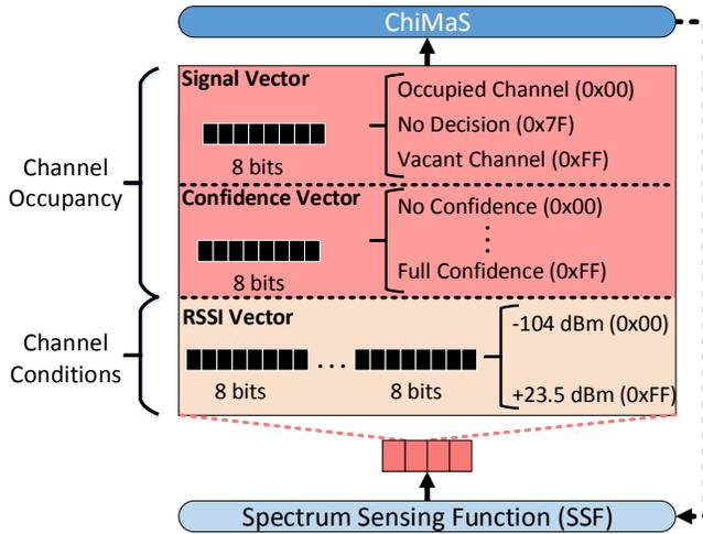
Fig. 2. GCL data structures
