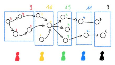
Assembly line worker assignment and balancing problem (ALWABP, Miralles et. al 2005).
