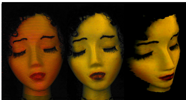
Figure 1. Picture of a dummy head showing projected laser stripes (left). A photograph of the dummy's face used for texturing (center). Reconstructed texture-mapped model (right).
