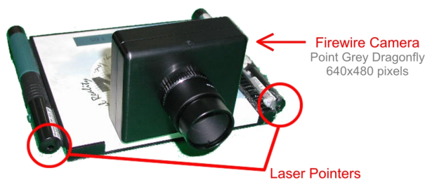
Figure 1: Prototype of the scanner for computing box dimensions.
