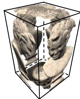
Figure 13. Object represented by six relief textures associated with the faces of a bounding box.
