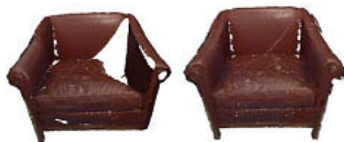
Figure 2: (Left) Chair extracted from the range image shown in Figure 8. Notice the existence of big holes due to occlusion. (Right) Symmetry-based Reconstruction (after [21]).
