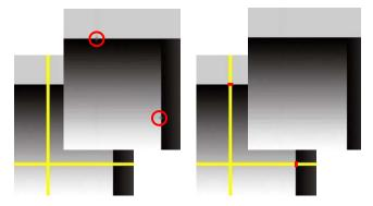
**Fig. 3.** The crossing lines define the inpainting domain (back left). Result of the isotropic diffusion introduces some blurring along high contrast edges (top left). User-added diffusion barriers (back right). Result produced with diffusion barriers (front right).
