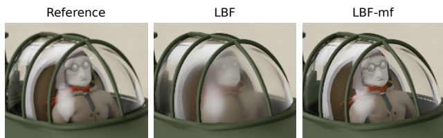
Fig. 4 Rendering using geometric features. Reference image (left). Overblurring on transmitted scene details caused by relying on features at the first intersection point (center). Using features from the first non-specular intersection allows the denoiser to preserve those details (right).
