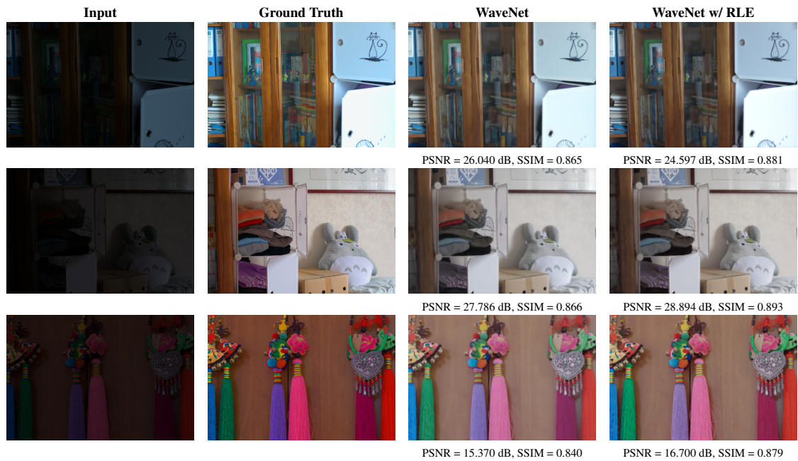
Figure 4.6 – Visual comparison of WaveNet results without and with the RLE block. As in Figure 4.5, the outputs are visually similar, demonstrating that the RLE block preserves the original enhancement quality while enabling additional user control.
