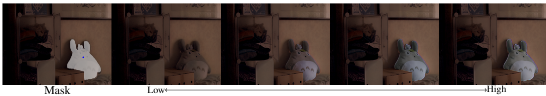
Figure 4.10 – Local enhancement control with the RLE block. The (highlighted) mask in the first image indicates the region targeted for adjustable enhancement. In the subsequent images, increasing the mask’s scaling value progressively brightens the selected region, while decreasing it darkens the region, leaving the brightness levels of surrounding areas unaffected. However, the boundary of the selected region tends to become overly bright as the enhancement level increases.
