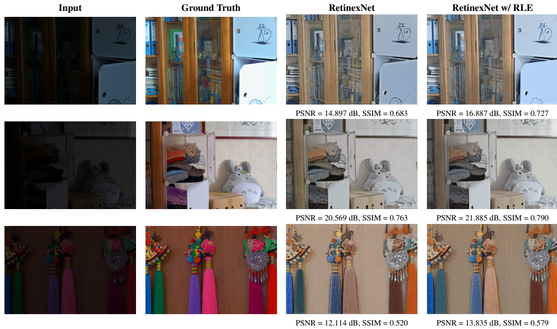
Figure 4.3 – Comparison of RetinexNet results without and with the RLE block. The results with the RLE block show a slight improvement, particularly in color saturation.
