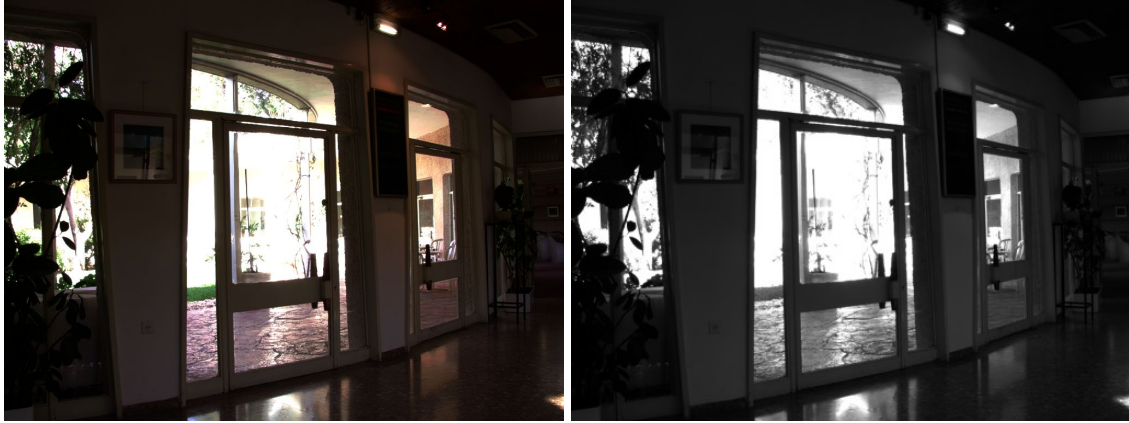
Figure 4.3: The unprocessed HDR RGB image (left) and its corresponding HDR luminance image (right), obtained by the evaluation of Equation 4.2 for each of the color pixels.
