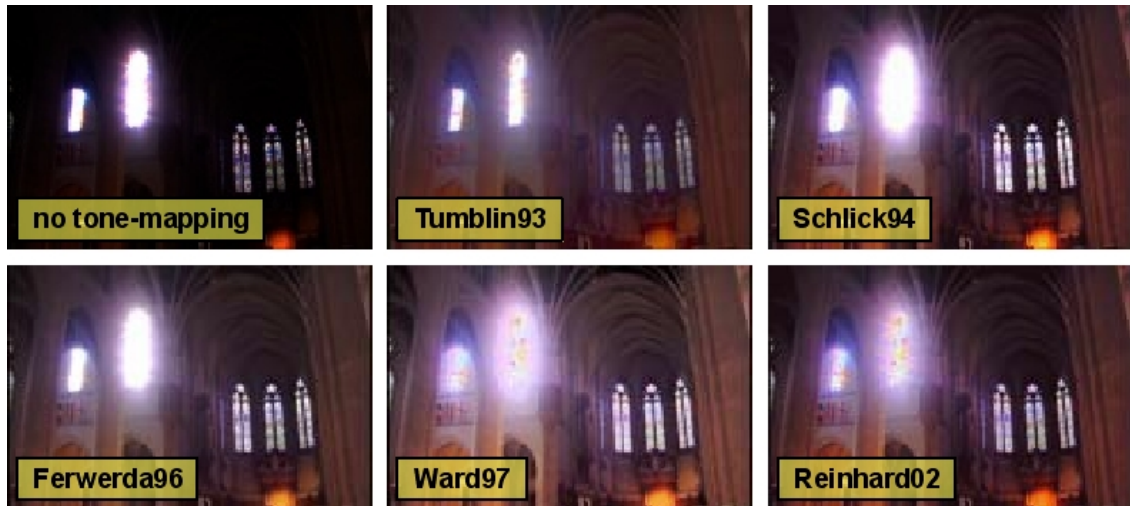
Figure 1.3: Example of a high dynamic range image (12 orders of magnitude) processed with various tone-mapping operators. Source: (REINHARD et al., 2002).
