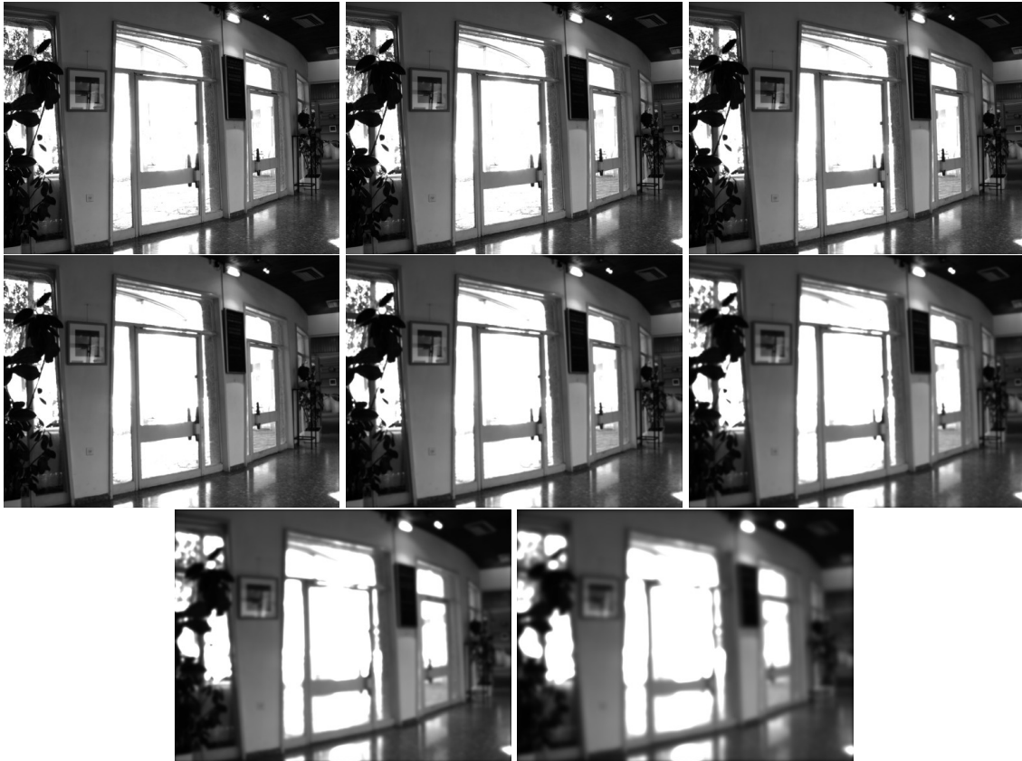
Figure 4.8: A set of Gaussian-filtered images from the relative luminance from Figure 4.4, according to Equation 4.9. The kernel sizes are, from left to right, top to bottom, 1, 3, 5, 7, 11, 17, 27 and 43, respectively.
