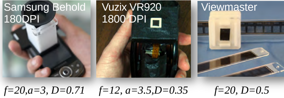
Figure 3.16: Three of the first prototypes: (left) cell phone, (center) high-resolution display, (right) View-Master. Variables f and a are measured in mm while D is in diopters.
