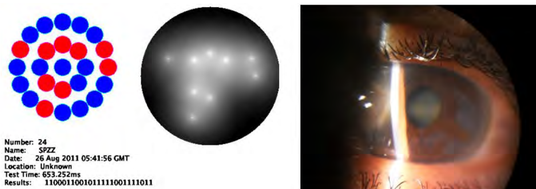
Figure 4.15: Comparison of CATRA results against the best slit-lamp picture of the captured dataset. Red circles indicate a covered subaperture. Although one could qualitatively compare the results, the lack of high-quality images of the cataract challenges a proper validation of the device.
