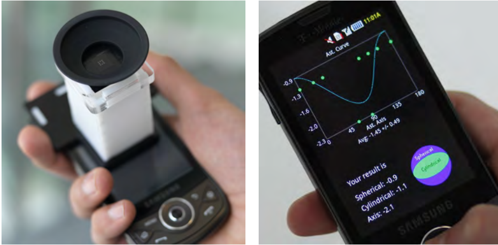
Figure 1.2: This thesis proposes two new patient-centric subjective methods to measure optical parameters of optical system. In this prototype, the cell phone clip-on (left) creates a limited light-field display designed for measurement of refractive errors in terms of spherical, cylindrical and axis of astigmatism (right). Photo by Jonathan Williams.
