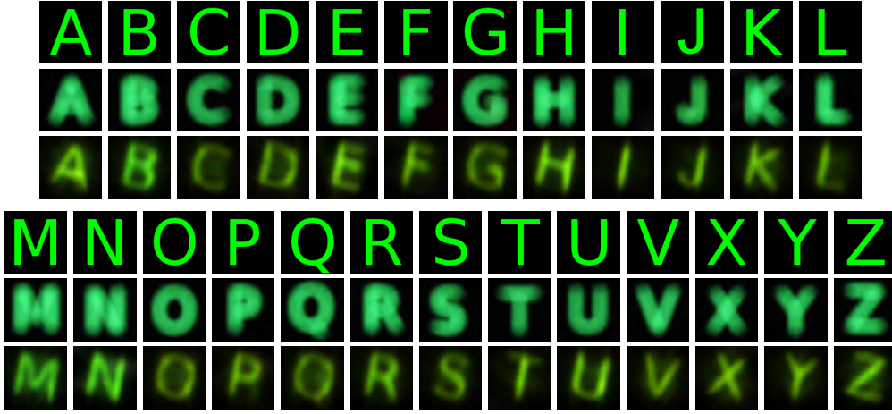
Figure 5.10: (top) Input images to the tailoring process. (middle) Simulated perception by a presbyopic subject of the respective target letters using a regular display. (bottom) Observation of the respective pre-distorted target letters but shown by the tailored display for the same presbyopic aberration. Subject's closest focal point is at 1.6D ( \approx 60cm , behind the display). The camera is placed 38.5cm away from the display. p = 28mm , m = 10.7mm , a = 70mm . Images are 1.41mm tall on the retina, reaching \approx 12.6mm on the virtual image plane. The pixel pitch at the virtual image is 0.125mm ( 0.69 arc minute resolution). In the trial runs, hardware misalignment produced slanted letters.
