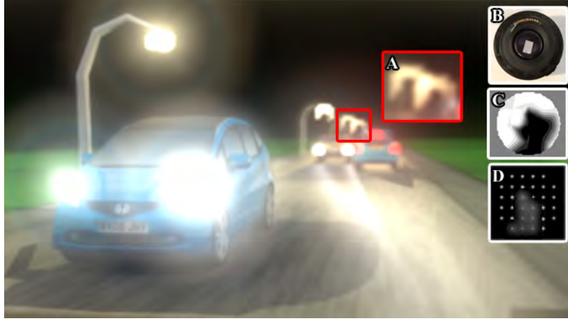
Figure 4.8: Rendering features using measured PSFs from a simulated cataract on a DLSR camera: (A) “Bokeh” effect, the cataract shape projected from out-of-focus bright light sources; (B) picture of the simulated cataract; (C) the estimated attenuation map; (D) the estimated PSF map; Cataract spots scatter light, generating large glare patterns. Depth information captured from the z-buffer. Camera aperture of 4mm .
