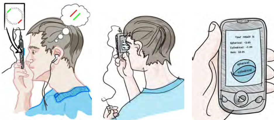
Figure 3.1: Can a person look at a portable display, click on a few buttons and recover his refractive fidelity? NETRA combines inexpensive optical elements, programmable display and interactive software components to create the equivalent of a parallax barrier display that interfaces with the human eye. This platform creates a new range of interactivity for measuring optical parameters of the human eye, such as refractive errors, focal range, and focusing speed.
