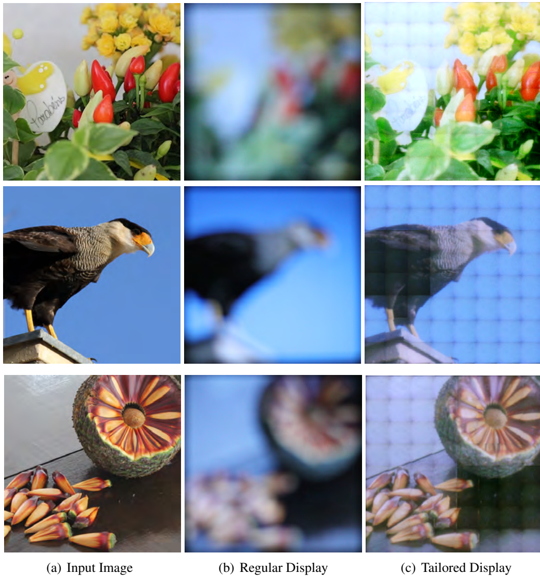
Figure 5.15: Input images (a) and how they are perceived on a tailored display by a farsighted subject (c). For this experiment, the HMD prototype was placed t = 20cm from the camera which is serving as the eye in this setup. The camera simulated a subject whose closest focal point was j = 50cm (subject using +3D lenses). Picture (b) shows how the subject sees the input image (a), with same size, at the same distance on a standard monitor. Since the setups have small spatial resolution, an array of LCDs is mimicked by changing the displayed image to cover a bigger "retinal" area. (c) is in reality a collage (sum) of 64 combined square patches which create a 3.4 arc-minute image on the retina (each patch = 0.425 arc minutes). The blue channel of (c) was adjusted to 75% of its captured intensity to remove prototype light leaking.
