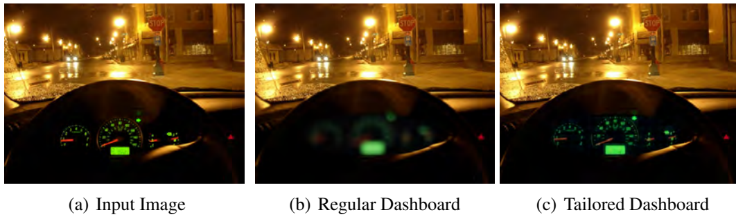
Figure 1.5: Difference in the view of a presbyopic subject when driving using a regular display (b) and a tailored display (c) on the dashboard of the car. (a) how an emmetrope would see the same view. Picture (b) shows how the subject sees the dashboard of (a) without wearing correction. The tailoring display restores visual acuity without needing eyeglasses or contact lenses. The dashboard of (b) is a photograph with a presbyopic camera looking at a regular display and (c) is a photograph using a presbyopic camera on a tailored display.
