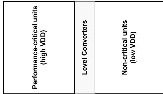
Figure 2.6: Two-level multiple static supply voltage scheme.
