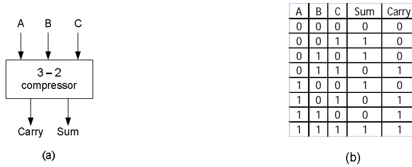
Fig. 4 – (a) 3-2 adder compressor. (b) Truth table for the 3-2 adder compressor.
