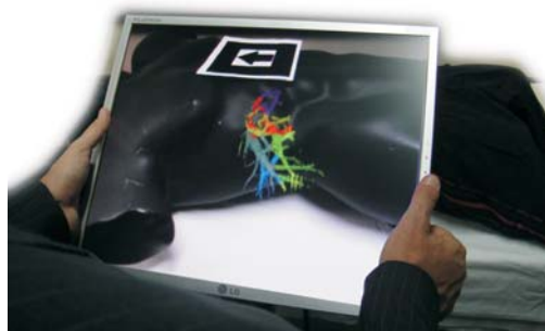
When an object of interest, e.g. a patient, is focused, their internal structures are rendered according to the angle and position of the participant.
