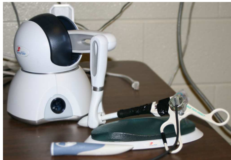
Figure 2. The PHANTOM Omni TM haptic interface device with surgical tool interface.
