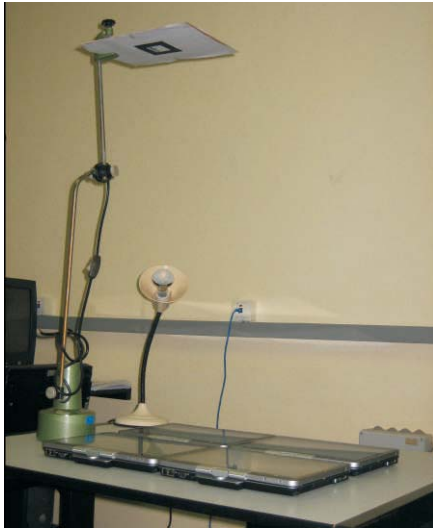
Figure 3. The marker positioned above the tablets, allowing capture by the web cameras.
