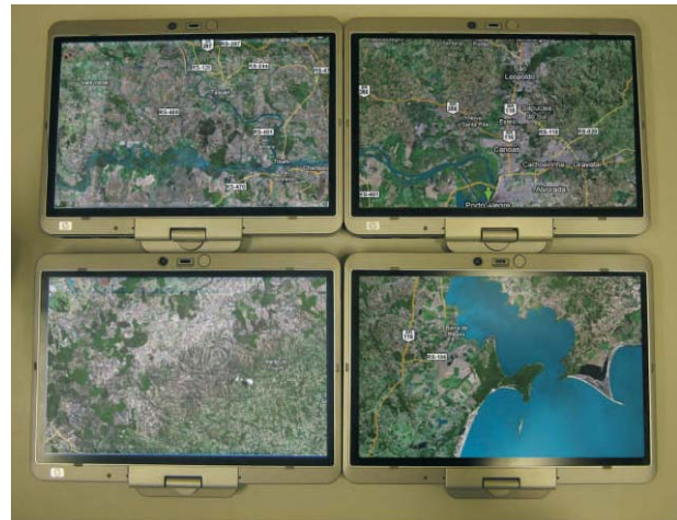
Figure 1. Arrangements with four tablets PCs, allowing to display an image of up to 2560 x 1600 pixels.
