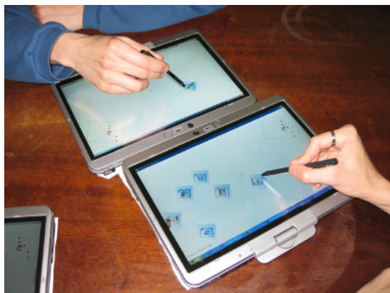
Figure 1. Proof-of-concept prototype of an application for file exchange: multiple users can drag and throw files to each other's workspace
