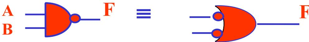
$$F = \overline{\overline{A} + \overline{B}} = \overline{\overline{A \cdot B}}$$
