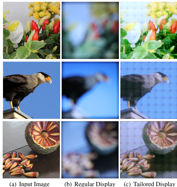
Figure 12: Input images (a) and how they are perceived on a tailored display by a farsighted subject (c). The HMD prototype was placed t = 20cm from the eye (camera). The camera simulated a subject whose closest focal point is j = 50cm (subject using +3D lenses). Picture (b) shows how the subject sees the respective image on (a), with same size, at the same distance in a standard monitor. Since our setups have small spatial resolution, we mimicked an array of LCDs by changing the image being displayed to cover a bigger "retinal" area. (b) is a collage (sum) of 64 square patches which create a 3.4 arc-minute image on the retina (each patch = 0.425 arc minutes). The blue channel of (c) was adjusted to 75\% of its captured intensity to remove prototype light leaking.
